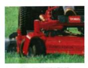
PRO RESULTS EVERY TIME TURBO FORCE® 5.5" deep cutting decks feature 18,500+ ft./min. blade tip speed and nearly 1/4" thick heat-treated steel blades.
